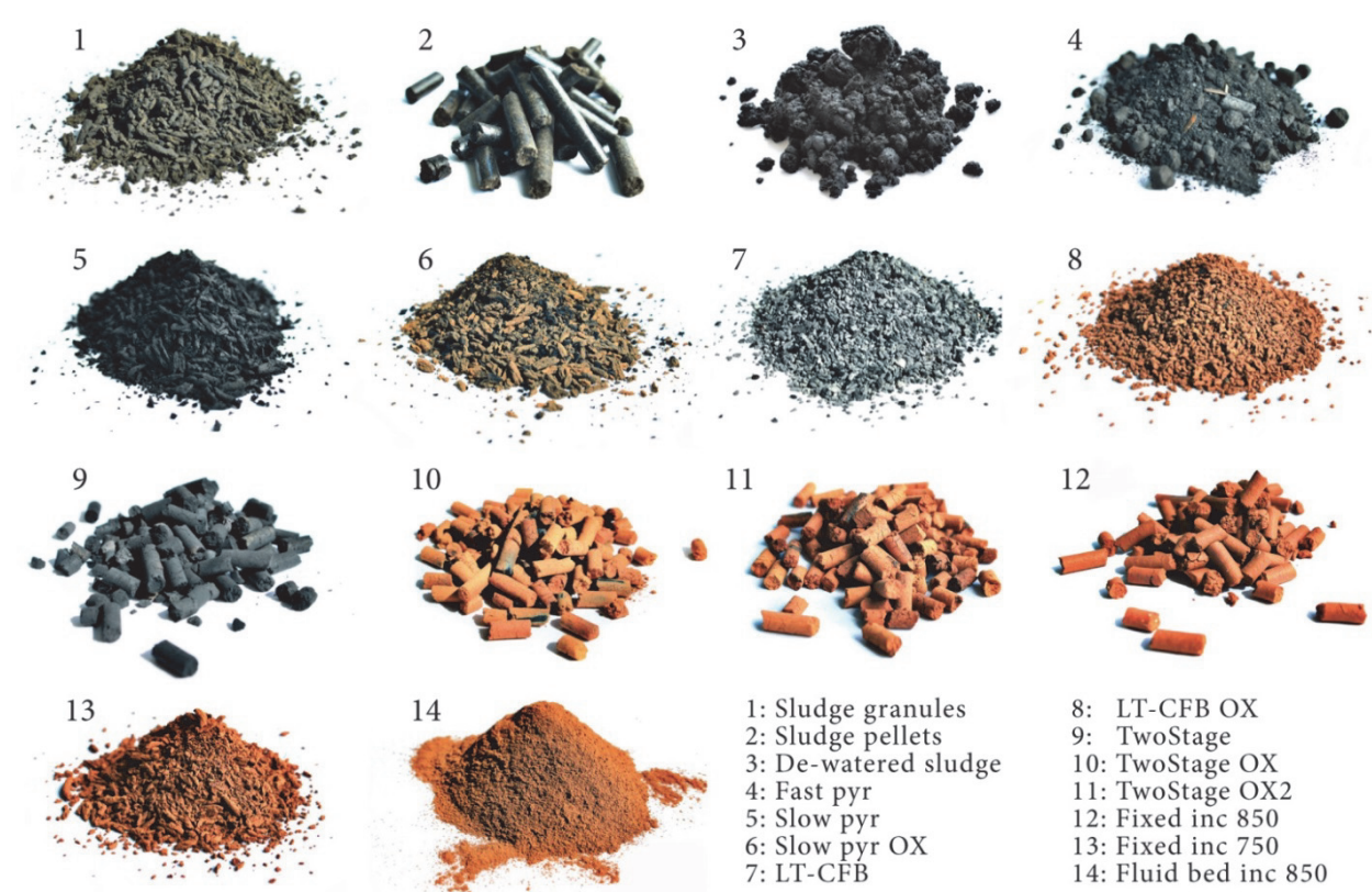
Figure 33: Pictures from the CPSE study of sludge fuel variants (1-3) obtained from the Danish WWTP Bjergmarken Renseanlæg in Roskilde as well as of ash and char substrates from pyrolysis (4-5), gasification (7,9), and incineration (12-14) of the sewage sludge samples. Post oxidized samples of slow pyrolysis char (6), LT-CFB bottom ashes (7) and TwoStage gasifier ashes (10-11) were also included in the study [4]
