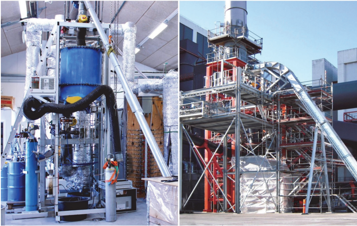
Figure 6: Existing LT-CFB gasifiers. Left: Pilot scale gasifier with a thermal capacity around 100 kW used by the Technical University of Denmark and located at Risø near Roskilde, Denmark. Right: Demonstration scale gasifier with a thermal capacity of 6 MW located at Asnæs Power Plant in Kalundborg, Denmark [62].
