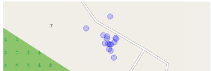
Fig. 4. Sample showing the error in precision typically observed in GPS measurements.
