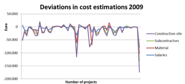
Figure 1. Deviations in cost estimations for the projects 2009 distributed between the main cost elements
