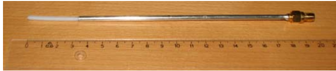
Fig. 3. The antenna element. (a) The measured scattering parameter S_{21} of the antenna immersed in an 80 % - 20 % glycerin-water solution. (b) Photo.
