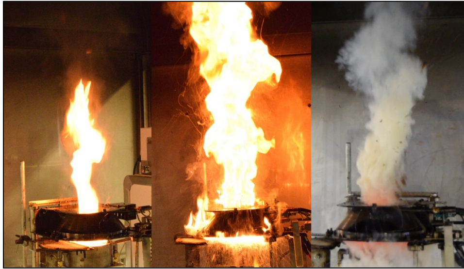
Figure 4.30. Regular burning (left), boilover (middle) and vapor explosion after the fire extinguished (right) of emulsified DUC (40/40) in the cone setup with an incident heat flux of 50 \text{ kW/m}^2 .
