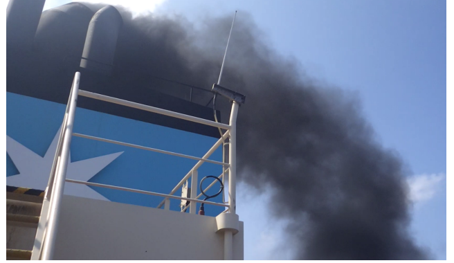
Figure 13: Exhaust smoke level with PI controller during engine speed step. Thick black smoke is emitted for 45 seconds.
