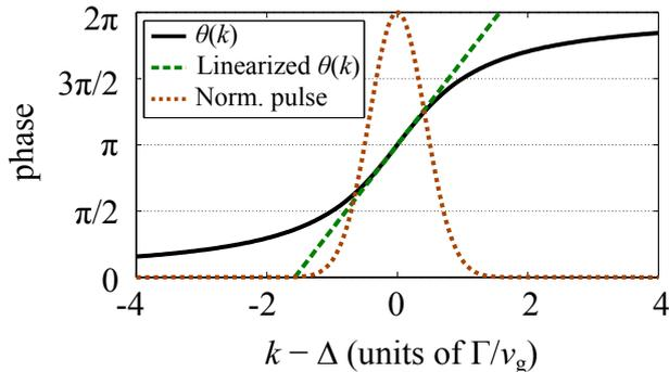
FIG. 2. Phase  $\theta(k)$  acquired by a single-photon wavepacket component with moment  $k$  propagating in a chiral waveguide scattering on a lossless resonant emitter (black solid line), together with a linear approximation, see Eq. (8) (green dashed line). By comparison, the spectrum of a resonant Gaussian wavepacket with spectral FWHM of  $\sigma = \Gamma/v_g$  is shown (orange dotted line) with a scaled intensity to match the plotting window.
