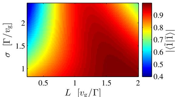
FIG. 3. Overlap between the ideal and scattered state for logical inputs  $|1_c\rangle|0_s\rangle$  or  $|0_c\rangle|1_s\rangle$  as a function of the additional optical length of the ‘0’ arms,  $L$ , and the input spectral width  $\sigma$  defined in Eq. (9).
