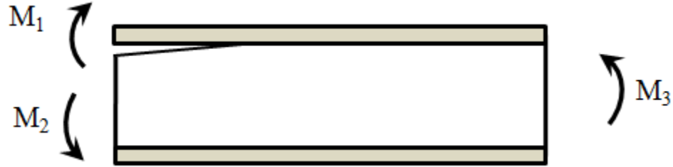
Figure 1. DCB-UBM specimen loaded with edge moments
