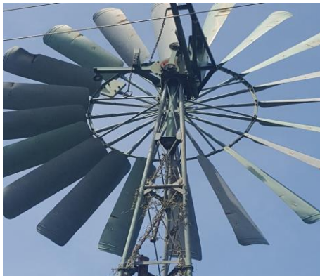
Photo 4: Mechanical wind pumps. Most of the systems have been replaced by solar systems
