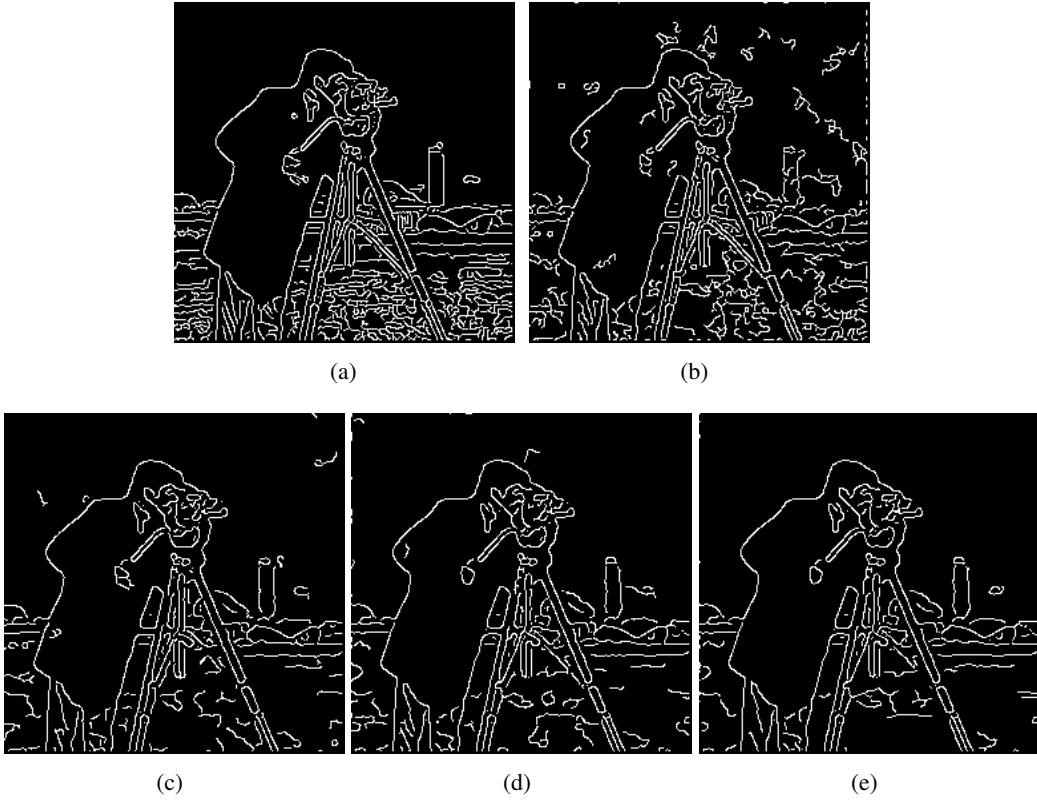
Figure 3. Edge maps of the fused images in Figure 2 by using the canny edge detector. (a) The original image; (b) FSGF [23]; (c) WFTV [20]; (d) FTVL1; (e) FTVL2.
