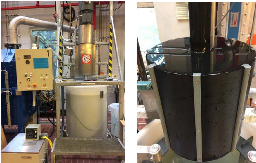
Figure 1: A pilot-scale rotary setup for drag resistance measurements (left) and the flexible rotor with six artificial welding seams on the periphery (right)
