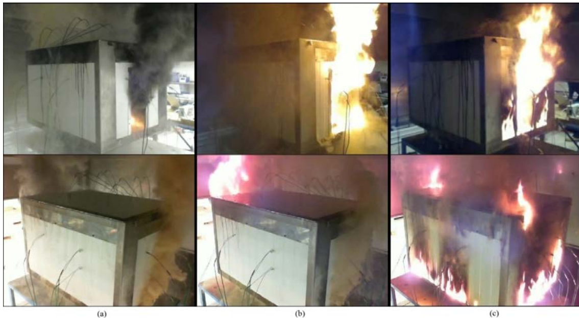
Fig. 13: Front (top row) and back (bottom row) view of PIR experiment 2. (a) 8.5 minutes after ignition. (b) After 9 minutes. (c) After 13 minutes.
