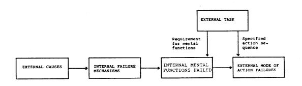
Fig. 4. Typical characteristics of an accidental chain of events including human malfunction.
