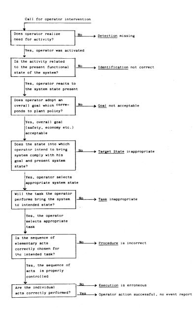
Fig. 7. Guide to identify the internal human malfunction from event analysis.
