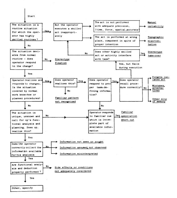
Fig. 8. Guide for event analysis to identify the mechanism of human malfunction.
