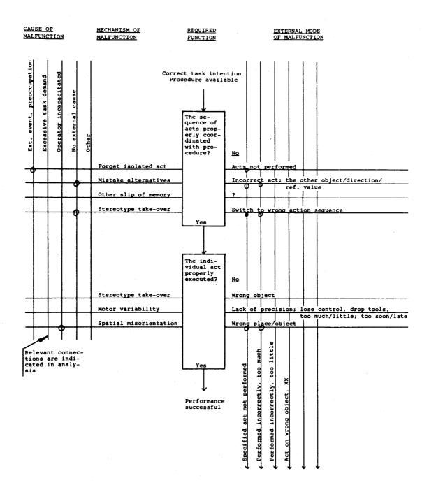
Fig. 10. Schematic format for prediction of error in action sequence. Will serve to generate fault trees in a failure mode and effect analysis. For illustrative purpose, only limited number of items in the different categories are included.
