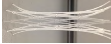
Figure 7.1: An example of a laser cut stent-base design after the initial heat treatment at 63°C
