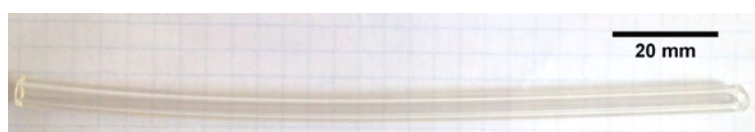
Figure 6.25: Extruded PLLA tube (16.5Fr)
