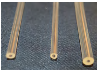
Figure 6.6: Extruded tubes with the outer diameters 13.2Fr, 10.2Fr and 16.5Fr
