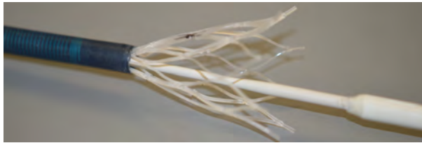
Figure 8.2: Loading of stent-base in delivery sheath
