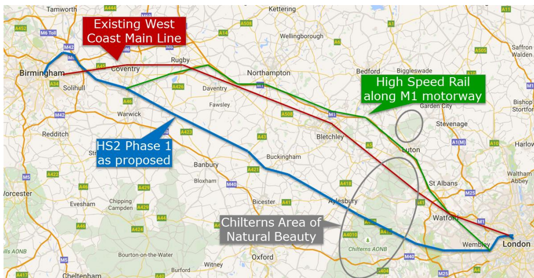
Figure 3: Alternatives along existing transport corridors considered for HS2 Phase I: Slower route along the M1 motorway (green); Upgrade of the existing West Coast Main Line (red).
