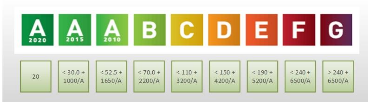
Figure 12 – Danish energy level scale for the EPC. The unit is kWh/m 2 a year, and A refers to the heated floor area in m 2 (DEA, 2016c). Graphic adapted from www.spareenergi.dk .
