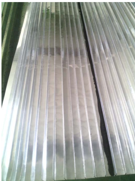
(c) The straight fins at the back of the absorber plate directly made by folding
