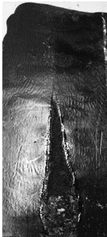
Fig. 5: Example of bitumen-reinforcement sample with fire retardant - after fire test.
