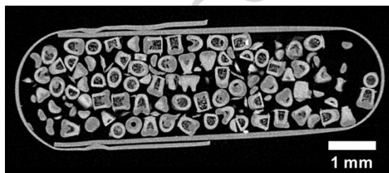
Figure 6: X-ray \mu\text{CT} image of a gelatine capsule filled with loaded and coated D-MCs.
