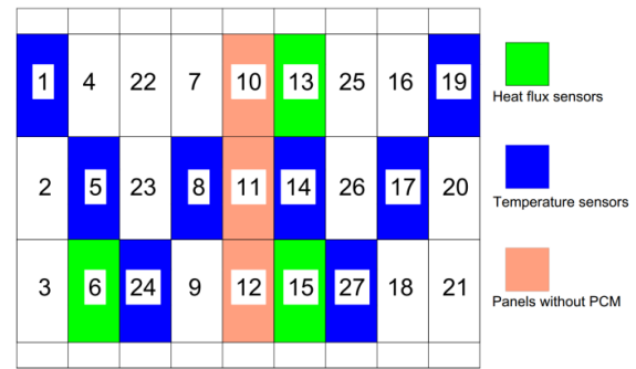
Figure 2: Sensors' location on PCM panels
