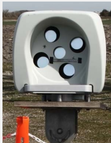
Avent 5-beam Demonstrator (5B-Demo): pulsed, step-staring
