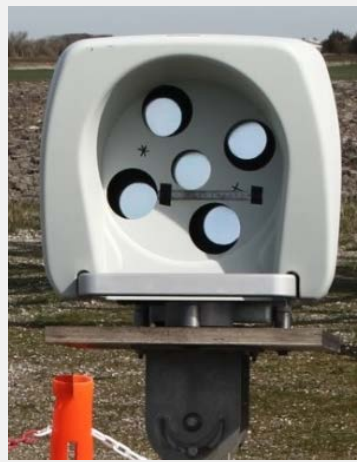
Avent 5-beam Demonstrator (5B-Demo): pulsed, step-staring
