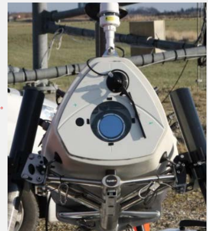
ZephIR Dual Mode (ZDM) continuous wave, conically scanning
