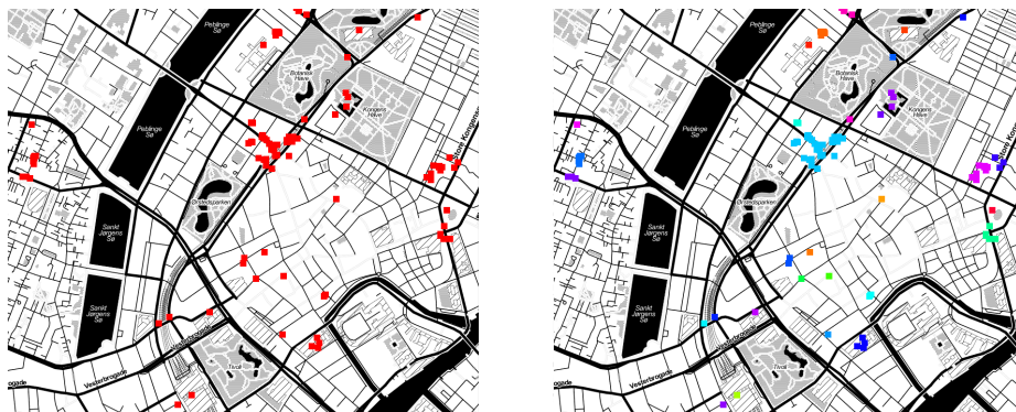
Figure 4.5: An example of identifying places as clusters of stops using density-based clustering (taken from Appendix I).
