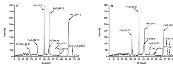
Fig. 3 XRD spectra patterns of composites of COP-1 (A) and COP-19 (B). Clearly visible is the Fe<sup>0</sup> peak at 44.9° 2θ, indicating the presence of ZVI contained within the composite matrices.
