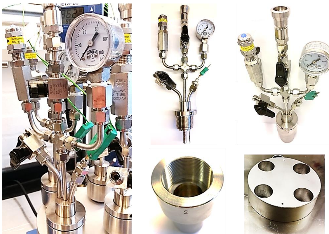
Figure 2.4: Images of mini high-pressure vessels
