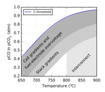
Fig. 3. A qualitative representation of the various restrictions on the possible operating window of a typical CO<sub>2</sub>-electrolysis stack. The y-axis refers to the measured outlet pCO of the stack. C-threshold refers to the Boudouard carbon deposition threshold.
