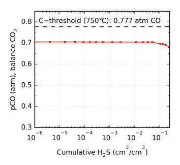
Fig. 6. The outlet gas concentration where carbon deposition was found to take place as found by means of iV-experiments is plotted against the cumulative  $H_2S$  flown into the cell. The x-axis unit refers to cm<sup>3</sup> of  $H_2S$  supplied per cm<sup>3</sup> of electrode.
