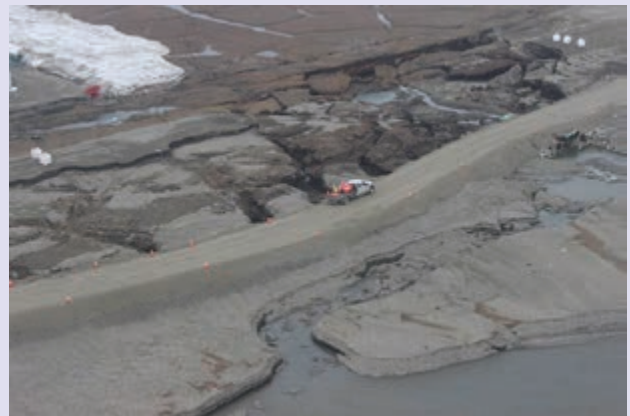
Figure 4.30 Area of thermokarst collapse near Deadhorse Airport as the flood water recedes (upper) and after thermokarst collapse and the start of reconstruction on 11 June 2015 (lower). Courtesy of AKDOTandPF.
