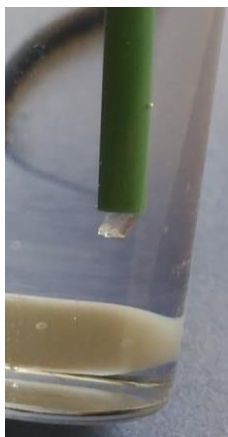
Figure 5.5 L-arginine crystal blocking the air injection point a few minutes after crash cooling.
