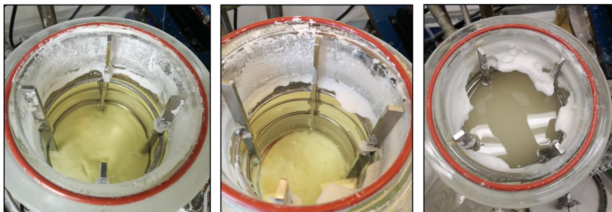
Figure 6.5 Crust formation at the top of the MSMPR crystallizer. Left: end of experiment A3 Middle: end of experiment A5. Right: end of the first attempt at experiment A6. None of the other experiments in this work presented this phenomenon.
