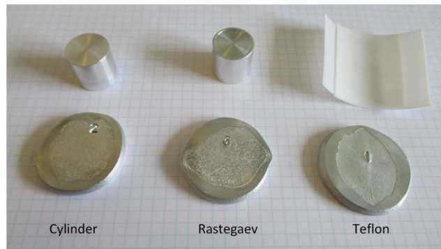
Fig. 2 Compression test specimens before and after deformation
