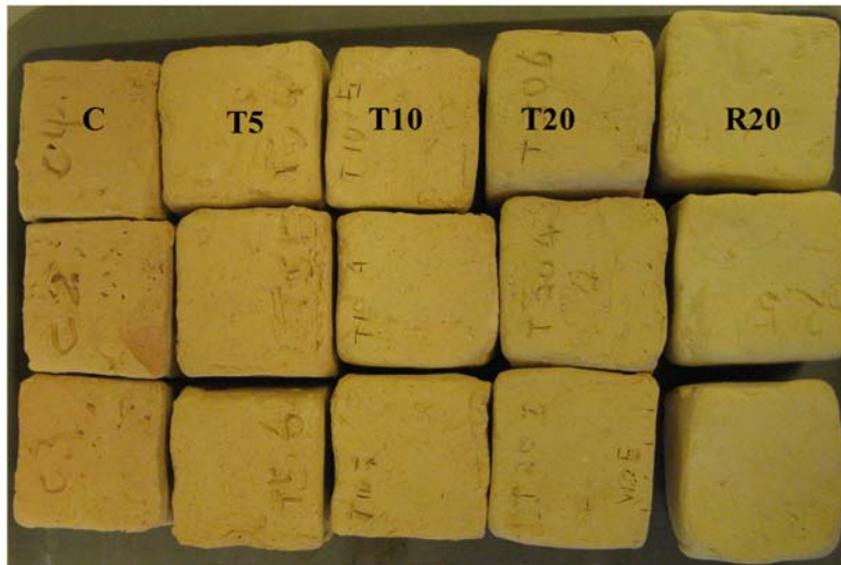
Figure 5: The appearance of the fired bricks. Notes: C – 100% clay, T5 – 5% treated MSWI fly ash; T10 - 10% treated MSWI fly ash, T20 - 20% treated MSWI fly ash; R20 – 20% raw (not treated) MSWI fly ash.
