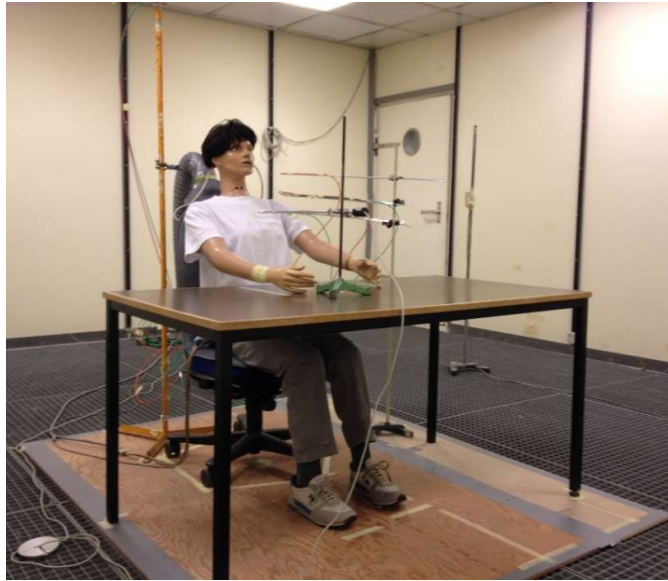
Figure 31: Room layout in the quiescent environment with the manikin dressed in summer clothing.
