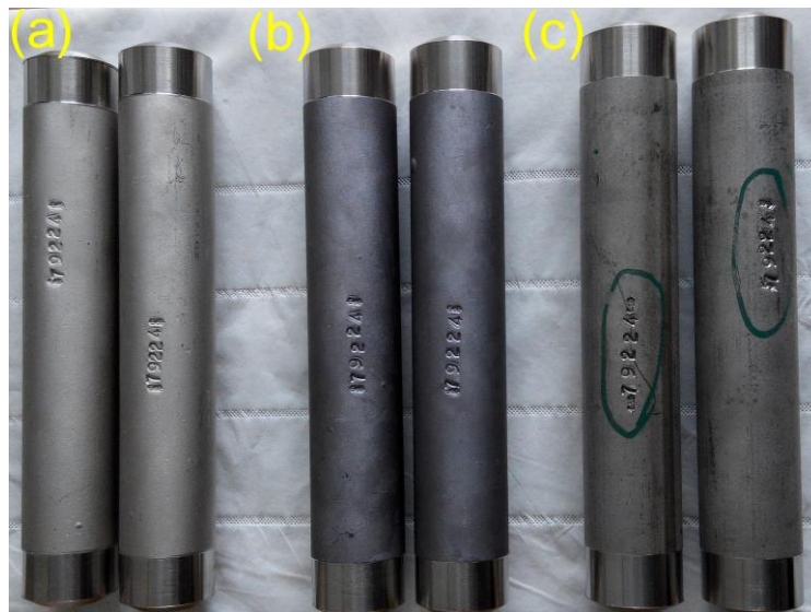
Figure 1. Morphology of (a) Ni coated, (b) Ni 2 Al 3 coated and (c) uncoated tubes
