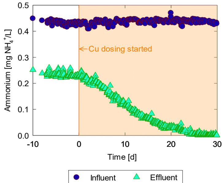
**Figure 1** – Ammonium concentrations in the influent and effluent of a biological rapid sand filter at a full-scale groundwater treatment plant in Denmark. Copper dosing through electrolysis was started on day 0. (Adapted from Wagner et al., 2016 a)
