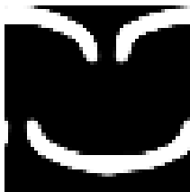
Figure 8: The unit cell resulting from optimizing with method 1 without symmetry constraints.
