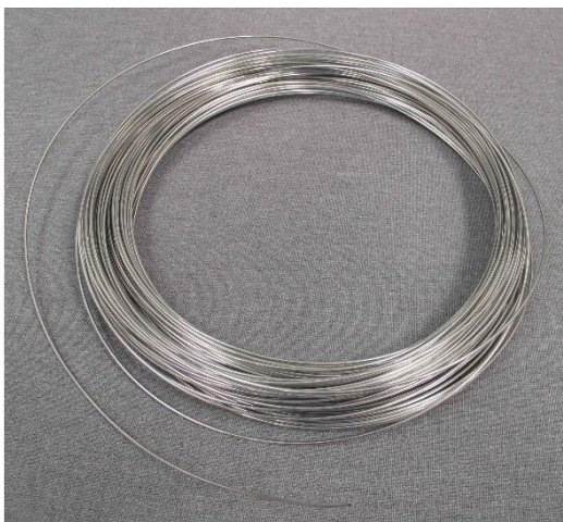
Fig. 3 Stock material; Form: coil, Material: EN-AW 1050A, Temper H14
