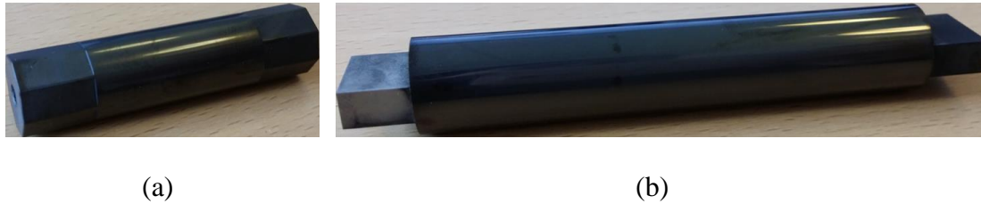
Figure 9.8: The Ø15 mm non-rotating a) upper and b) lower tool pins deposited with the double-layer DLC/Hyperlox® coating. Technical drawings are shown in Appendix G2.
