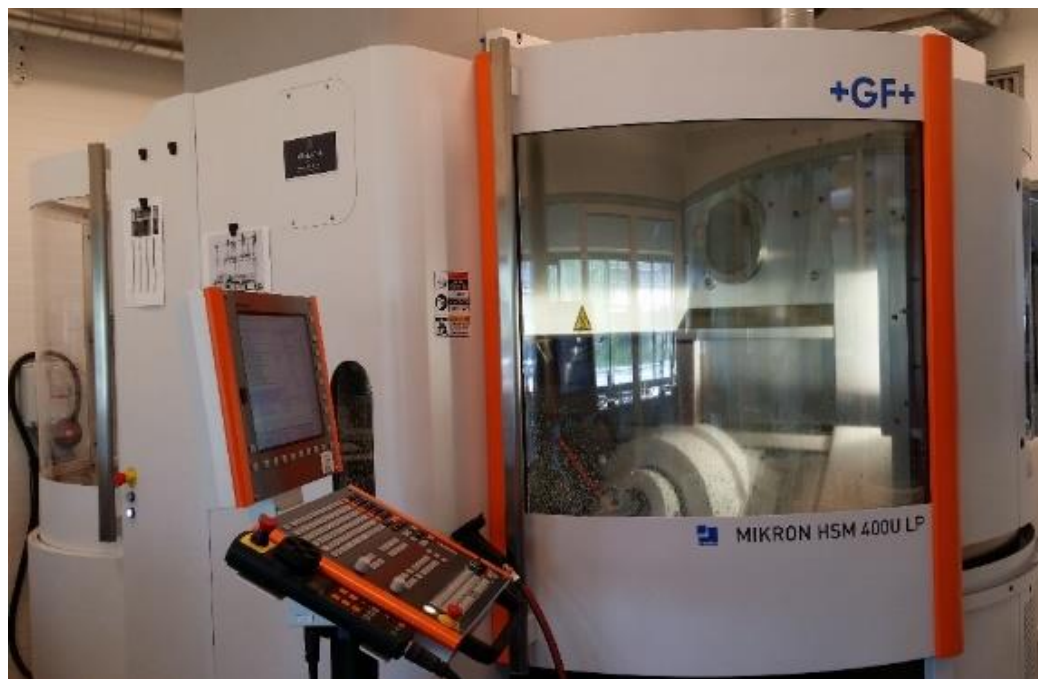
Figure 6.4: Five-axis high speed milling machine for machining the pockets.
