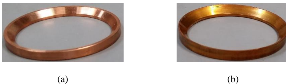
Figure 5.6: a) Copper ring before the test, b) ring after successful test, no extrusion at 550 MPa.
