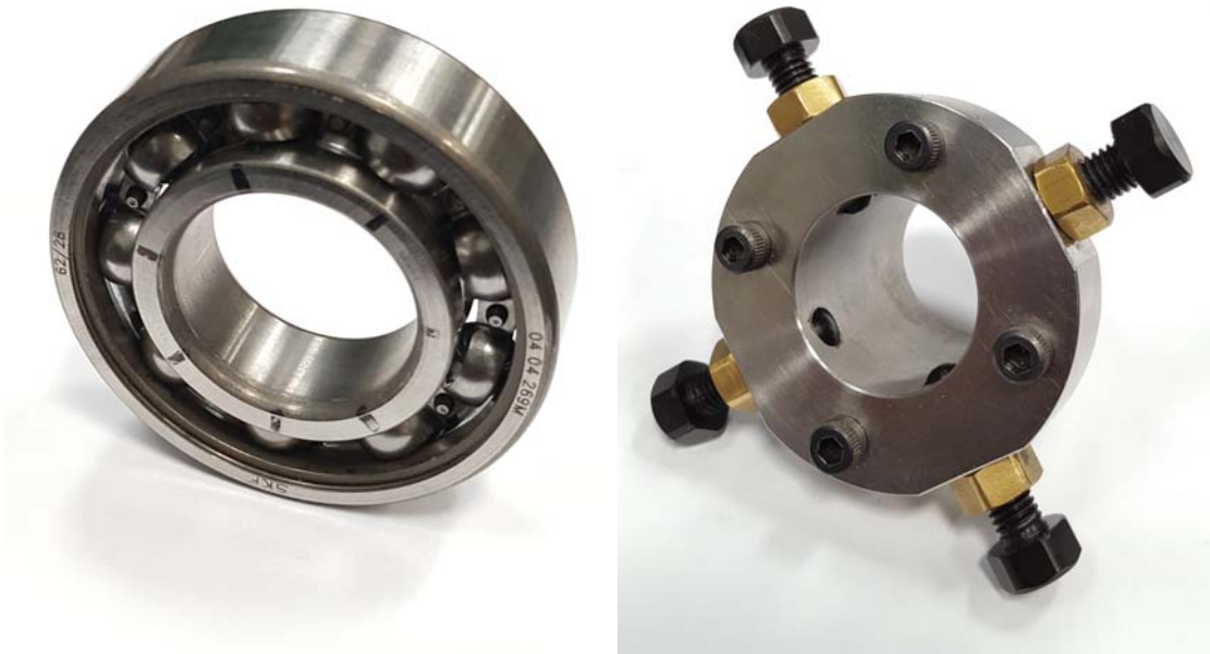
Figure 1.2: The ball and pinned bearings used for experimental test rig as the backup bearings.
