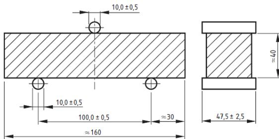
Fig. 4. Setup for three-point bending test (DS/EN-196-1-1, 2005)
