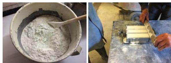
Fig. 3. Mixing and casting of prisms and cylinders
