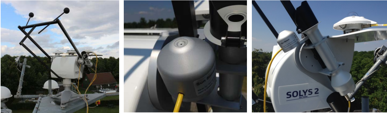
Figure 3: The SOLYS 2 tracker. On the top mounting plate, the solar radiation measurement instruments can be seen. On the left side of the tracker, the solar sensor and the pyrheliometer that measured the shortwave beam normal irradiance can be seen.
