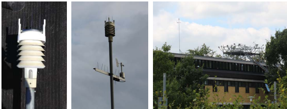
Figure 4: Weather station, type Vaisala WTX520. The weather station is mounted 6 meter above the roof of building 119.
