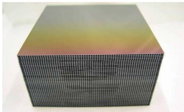
Fig. 2. SPO stack with 45 mirror plates
