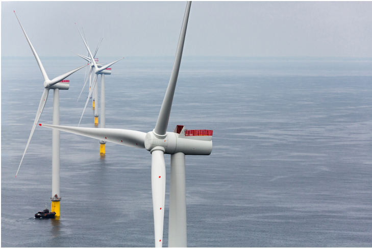
Figure 2.2: Siemens 6 MW offshore turbines in operation. This is a direct-drive design where the drive train consists only of a single rotor bearing and a low-speed synchronous generator. Notice the heli-hoist platform mounted on each turbine which allows crew transfer by helicopter.
