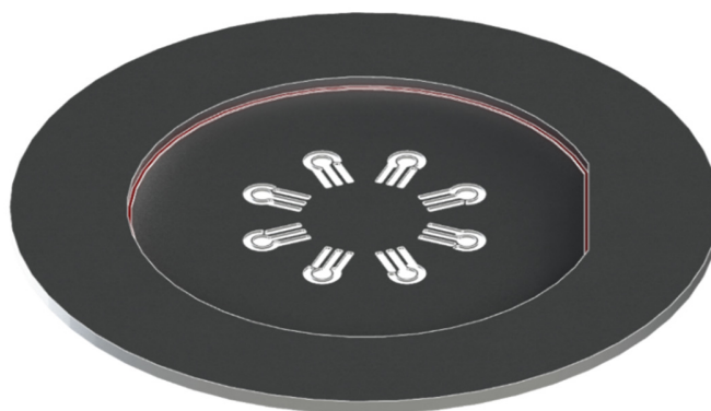
Figure 24. Schematic showing micro-milled holder with inbuilt shadow mask and room for holding 4-inch wafer with nanostructures.
