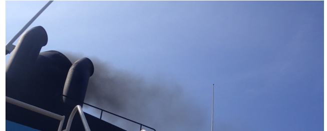
(b) Y_{LA}+AFF . The smoke level is reduced compared to the PI controller but still visible.
