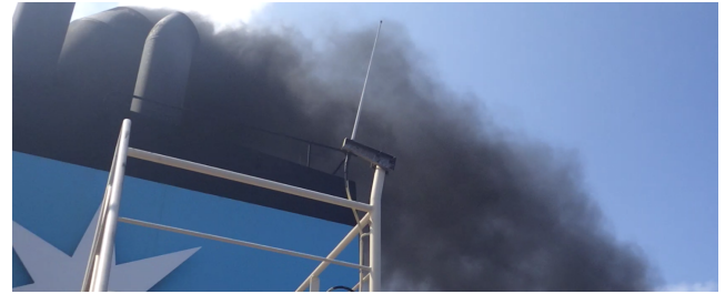
(a) Y_{LA}+PI . Thick black smoke is emitted for 45 seconds.
