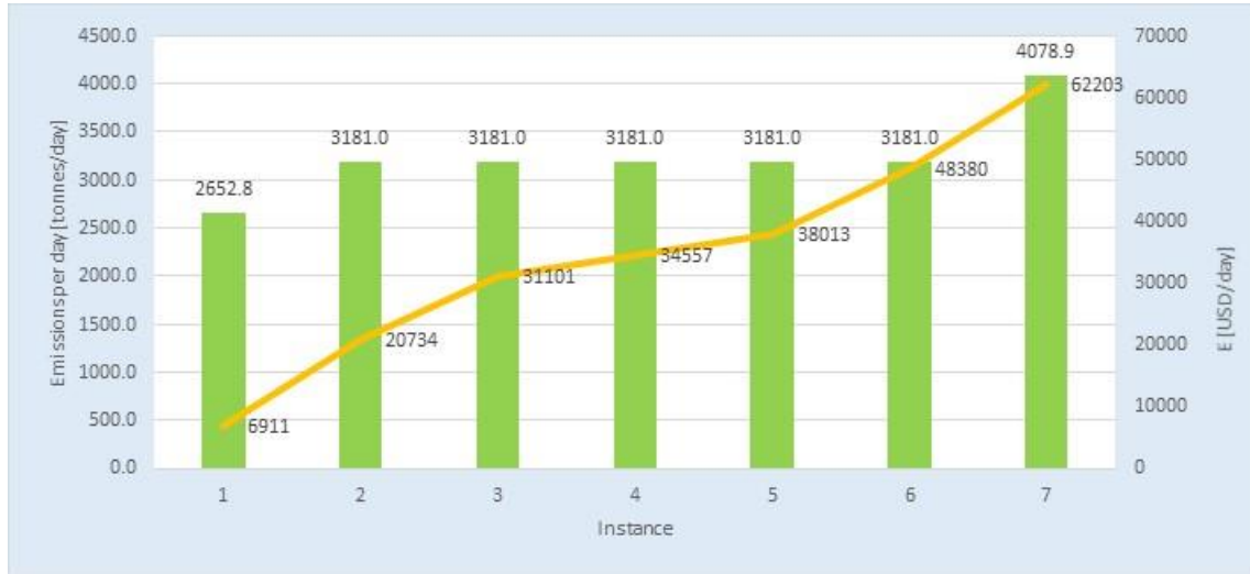
Fig. 6: Fixed service period scenario, effect of the daily operating fixed costs on daily CO 2 emissions (route AE2)
