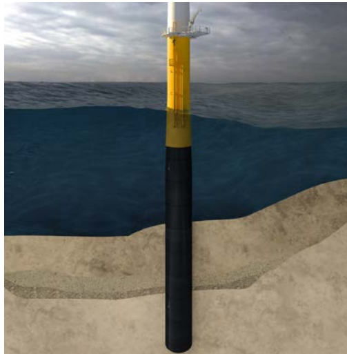
Figure 1. Conceptual sketch of the MP foundation incl. a TP joined to the bottom of the WTG tower. The top of the monopile is joined to the transition piece and the bottom of the monopile is fixed in the seabed. Figure: © COWI A/S.
