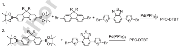
Fig. 37. Synthesis of copolymer based on benzothiadiazole, thiophene and fluorene, PFO-DTBT.
