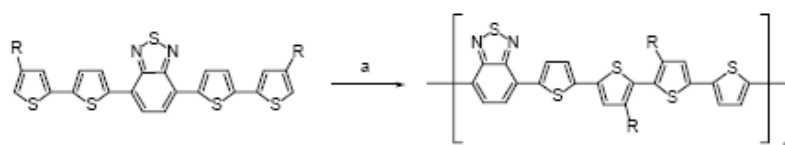
Scheme S5: Oxidative ferric chloride polymerization to give head-to-head copolymers of di-thiophene and benzothiadiazole, R= hexyl ( 27 ) or dodecyl ( 28 ). a: FeCl 3 , CHCl 3 .
