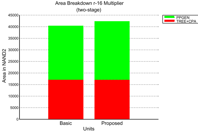
Fig. 9. Area breakdown for 2-stage pipelined multipliers.
