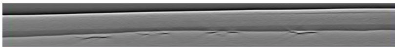
Fig. 6: Reconstruction using the algorithm in [45] of a large, solid-filled cylindrical vessel with crack simulations. The limited angle exterior data are for angles \varphi \in [0, 3\pi/4] and p \in [34.75, 36.75] cm. The picture is a quarter of the annulus graphed in polar coordinates (r, \varphi) (where Cartesian coordinate x = (r \cos(\varphi), r \sin(\varphi)) ). Angles \varphi \in [0, \pi/2] are along the horizontal axis and radius r \in [34.75, 36.75] on the vertical axis, with the inside at the bottom and the outside at the top. The outer boundary of the object is the dark curve near the top of the reconstruction. The scale in r is magnified so the cracks are easier to see.
