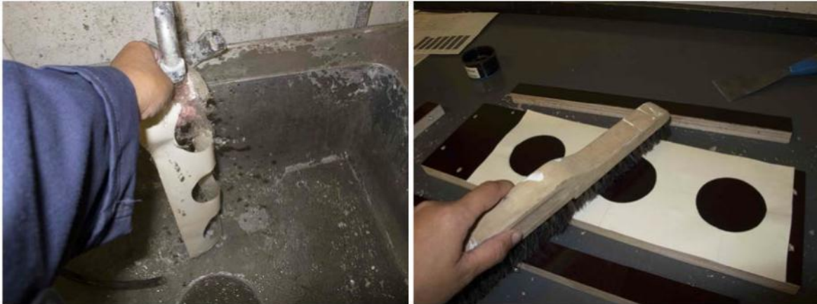
Fig. 1. The paper was moistened before it was Fig. 2. The wet paper glued to the base, placed on the base of the mould.
