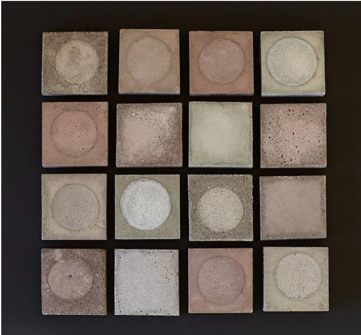
Figure 5.1 Mortar samples with different percentage of SSA and milled SSA
