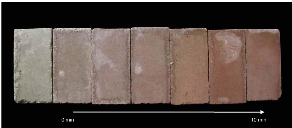
Fig. 3. Colour scale of moisturized mortar samples. The Grey colour of normal mortar gradually changes as the fineness of SSA particles increases. The first mortar sample to the left does not contain any SSA. The second sample contains un-treated SSA. Hereafter, the samples contain ground SSA of increasing fineness.
