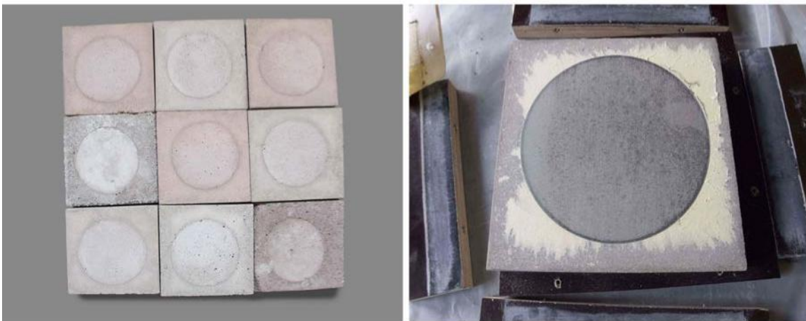
Fig. 5. Accentuation of colour displayed by the difference of rough and smooth surfaces. The circular parts are smooth and the surrounding areas are rough. Fig. 6. Paper stuck to the hardened concrete tile.
