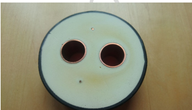
Figure 4: Double DH pipe system by Logstor.
