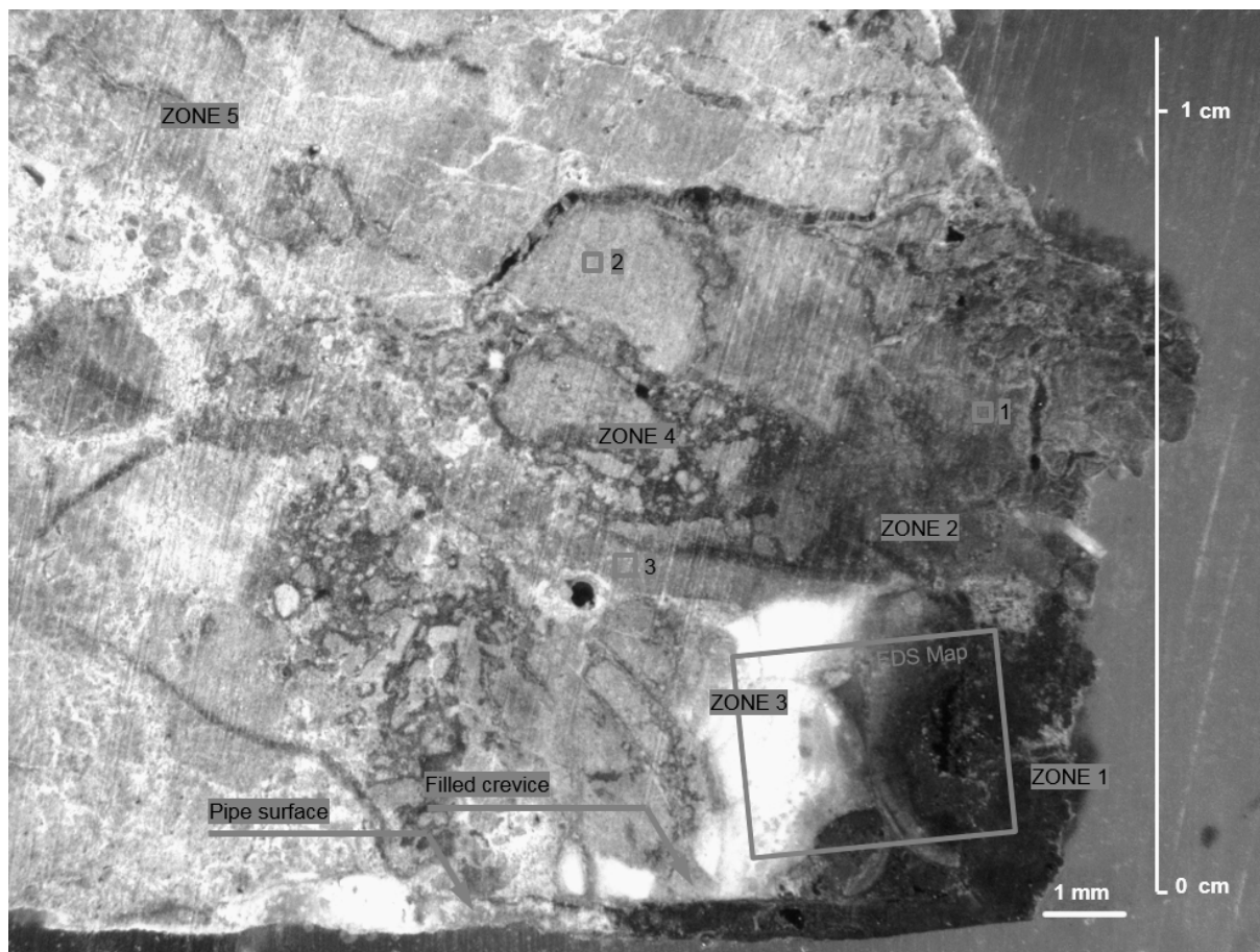
Figure 6. Cross-section of the stone-hard-soil close to the corrosion site in the lower right corner (0-1 cm), moulded in epoxy resin. Marked areas were investigated with EDS, see Figure 7 and Figure 8.
